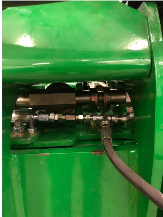
7. When installing the small cylinder ensure to install it on the side that has the most clearance.
