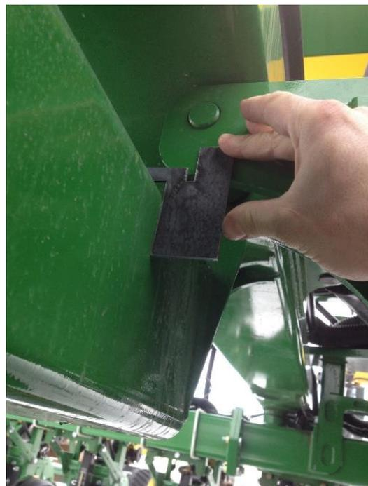
As indicated in the photo below, trace along the corner on the template shown with a red mark in the photo, this is the area where you will need to cut or grind away. The possibility of the tip bracket lining up with a bolt right at the roller mount isn't very likely but if happens to be the case then the green line in the template photo indicates the additional amount you will have to cut.
