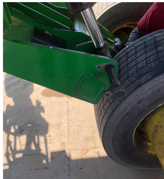
6. With axle assembly properly supported, remove lower axle mount castings on both sides. (See illustration)
