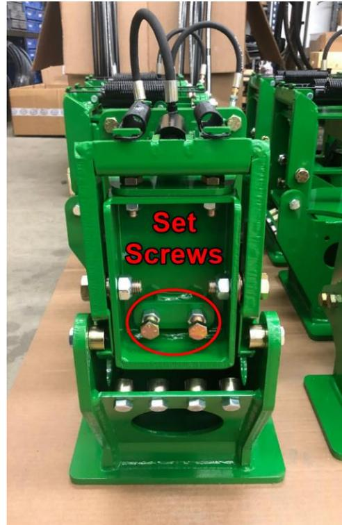
9. Once the bracket bolts, set screws and jam nuts are tightened down, row unit and row tip installation is completed.
