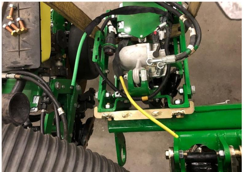
6. When tightening the fittings shown in the picture below ensure not to over tighten them as they may break. Tighten them to a snug fit to ensure no leaks.
