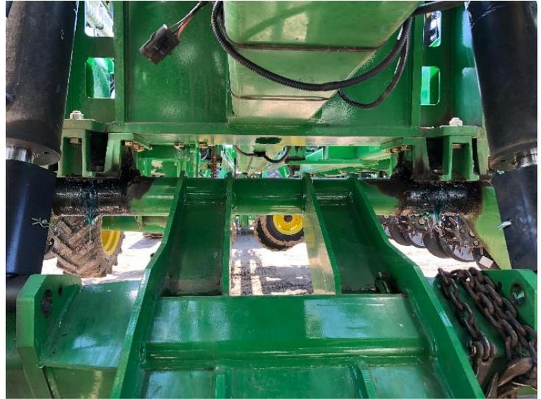
7. Lower assembly to the floor with proper restraint or lifting/lowering device.
