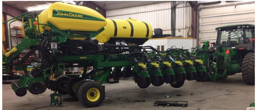
2. With planter weight supported on jack stands begin removal of the existing axle assembly.
