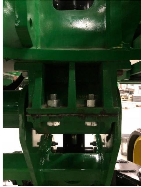
6. Insert flag pin through cylinder lift eyes and fasten retaining bolt on flag. On older DB planters the factory pin is too short, if your pin is not 10 inches of effective length a new one should have been included with your kit. **MAKE SURE YOUR PIN IS LONG ENOUGH TO GO THROUGH ALL THE PLATES ON THE LIFT ARM!!!** On a DB44 planter we use a plain pin and trunnion blocks bolted into the lift arm on the track axle instead of a flag pin.
