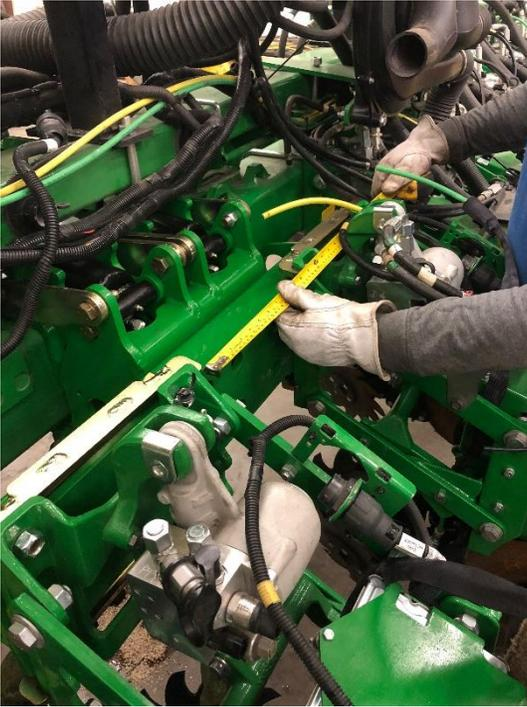
5. Once desired placement is achieved. Tighten all bolts on the mounting brackets starting with the top bolts and lock nuts.
