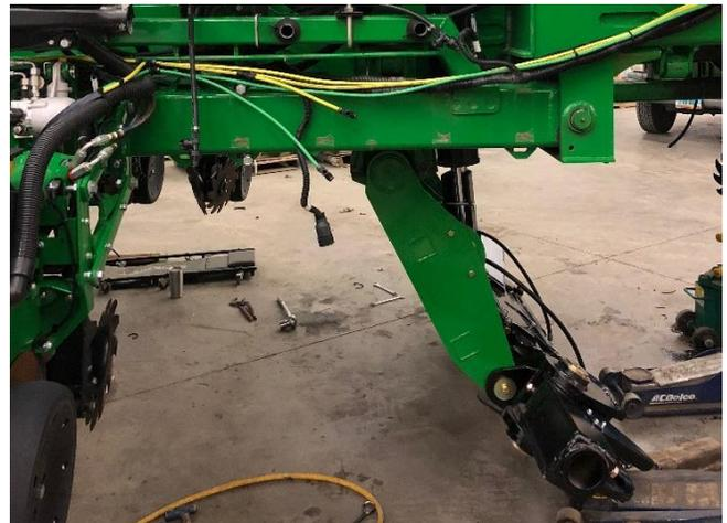
4. Align side to side to be sure lift cylinders line up with mounting tabs on axle assembly.
