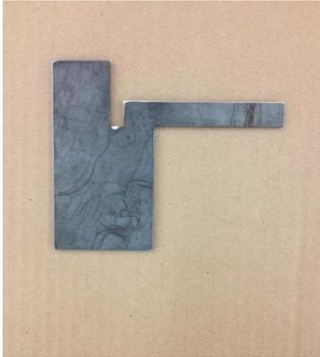
We have found some of the newer DB planter frames have less clearance in the bracket that mounts a roller. Use the gauge to see if your planter has enough clearance for the row tip to fit. With the planter folded up hold the template up to your roller brackets resting the long narrow part on top of the 7x7 tube and holding the template tight to the front side of the tube, see photos below.
