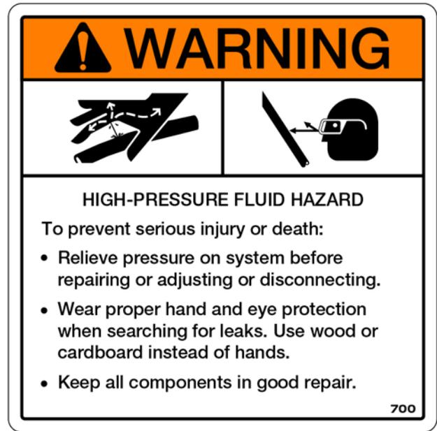
Hydraulic fluid that is escaping under pressure can have sufficient force to cause injury. Confirm all hoses and connections are always in good working order by looking over daily. Failure to do so may result in serious personal injury or death. Escaping hydraulic fluid under pressure may have enough pressure to penetrate skin causing serious injury. Avoid this hazard by relieving the pressure before disconnecting lines or servicing the system.
