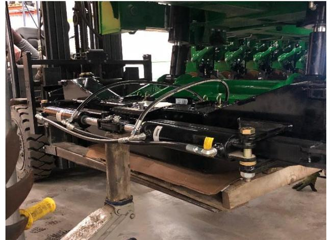
2. Begin installation of tracked axle assembly in reverse order of disassembly.
