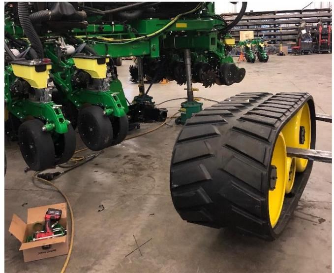
2. Line the axle pin and the slot in the axle up and slide the track onto the axle assembly. Be sure the bolt holes are lined up for easy installation of the bolt.
